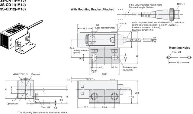
Note: Models numbers for Through-beam Sensors (E3S-CT61(-M1J)) are for sets that include both the Emitter and Receiver.
