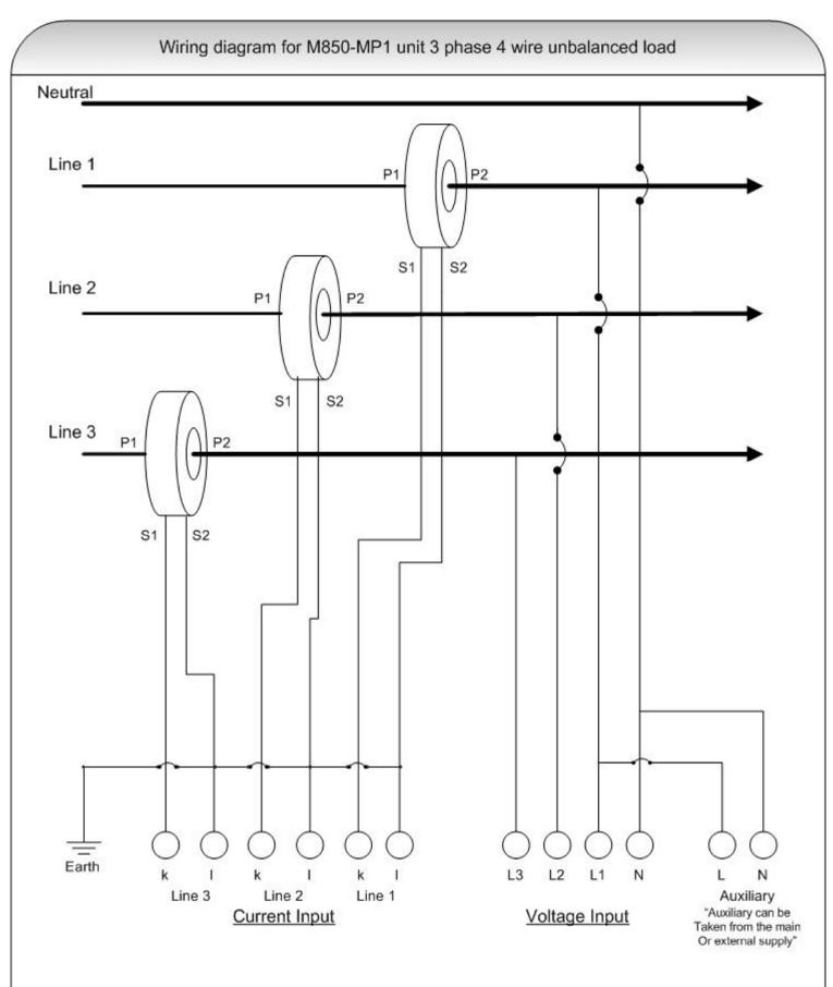
The above diagram is based on 3 phase 4 wire unbalanced load
