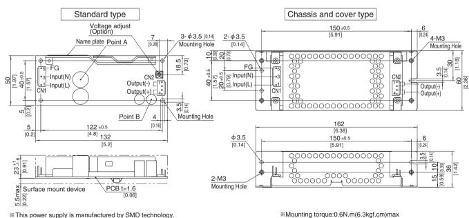
This power supply is manufactured by SMD technology. The stress to P.C.B like twisting or bending causes the defect of the unit, so handle the unit with care. Take care for SMD parts on the back to come in contact because of the vibration and not to break down.
