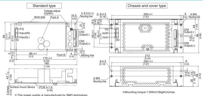
\* This power supply is manufactured by SMD technology. The stress to P.C.B like twisting or bending causes the defect of the unit, so handle the unit with care.
