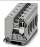
Feed-through terminal block, Connection method: Screw connection, Cross section: 1.5 mm<sup>2</sup> - 50 mm<sup>2</sup>, AWG: 16 - 1/0, Width: 16 mm, Color: red, Mounting type: NS 35/7,5, NS 35/15
