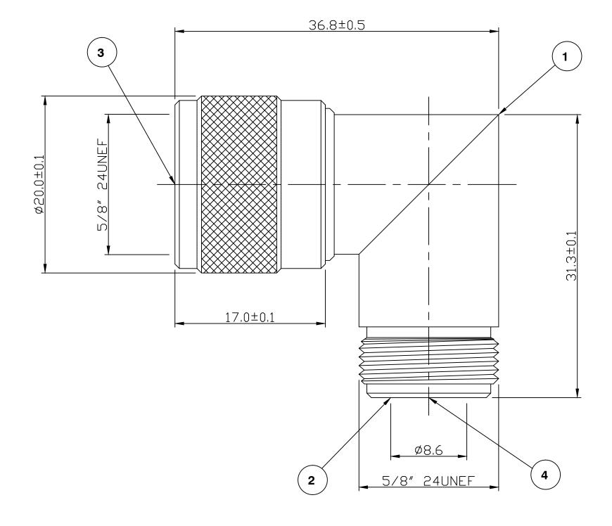
Nominal Impedance: 50 ohms Frequency Range: DC to 11 GHz
