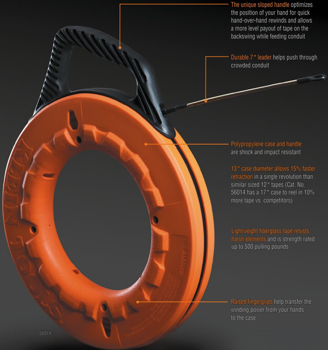
The unique sloped handle optimizes the position of your hand for quick hand-over-hand rewinds and allows a more level payout of tape on the backswing while feeding conduit
