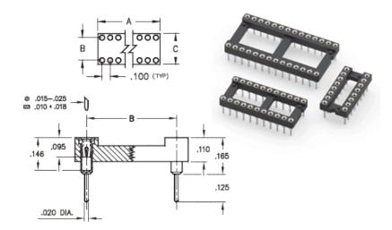
**Description:** DIP Dual In Line Socket Standard Solder Tail Open Frame Through Hole Plating Code: Shell Plating: 200 µ" Tin (matte finish) over 100
