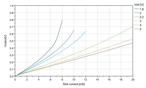
Figure 32-23. : I/O Pin Output Voltage vs. Sink Current (T=25°C)
