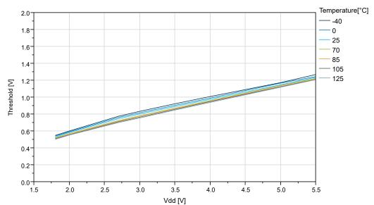
GPIO Input Characteristics Figure 32-16. I/O Pin Input Hysteresis vs. V<sub>DD</sub>
