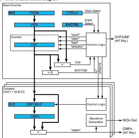
Figure 20-2. Timer/Counter Block Diagram
