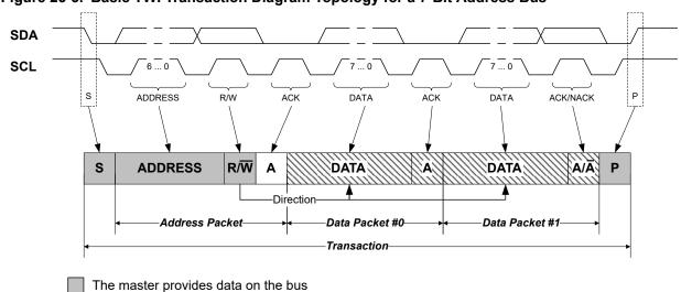
Figure 25-3. Basic TWI Transaction Diagram Topology for a 7-Bit Address Bus
