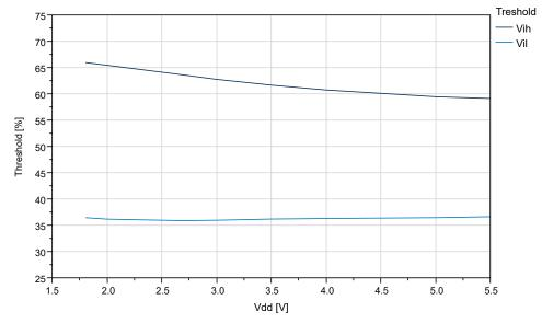
Figure 32-17. I/O Pin Input Threshold Voltage vs. V<sub>DD</sub> (T=25°C)
