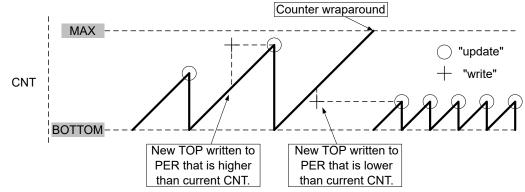
A counter wraparound can occur in any mode of operation when up-counting without buffering. This is due to the fact that the TCAn.CNT and TCAn.PER registers are continuously compared: if a new TOP value is written to TCAn.PER that is lower than current TCAn.CNT, the counter will wrap first, before a compare match happens.
