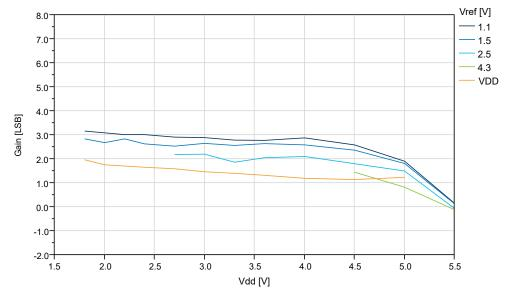
Figure 32-45. Gain Error vs.  $V_{DD}$  (f<sub>ADC</sub>=115 ksps) at T=25°C, REFSEL = Internal Reference
