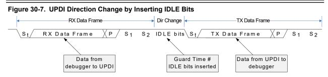
The UPDI Guard Time is the minimum IDLE time that the connected debugger will experience when waiting for data from the UPDI. Because of the asynchronous interface to the system, as presented in Clocks, the ratio between the UPDI clock and the system clock will affect the synchronization time, and how long it takes before the UPDI can transmit data. In the cases where the synchronization delay is shorter than the current Guard Time setting, the Guard Time will be given by GTVAL directly.
