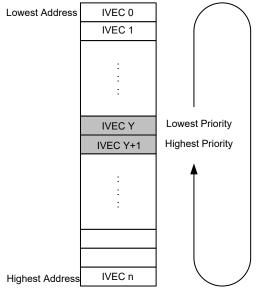
Figure 13-4. Static Scheduling when CPUINT.LVL0PRI is Different From Zero
