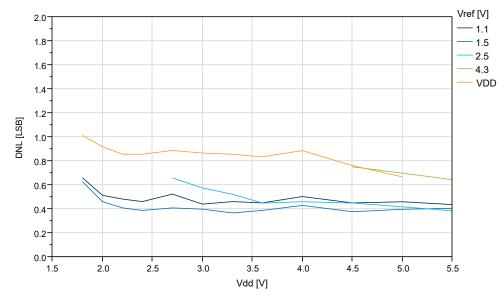
Figure 32-43. DNL Error vs.  $V_{DD}$  (f<sub>ADC</sub>=115 ksps) at T=25°C, REFSEL = Internal Reference
