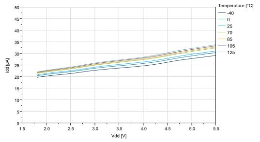
Figure 32-36. BOD Current vs. V<sub>DD</sub> (Sampled BOD at 125 Hz)
