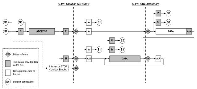
The number of interrupts generated is kept to a minimum by automatic handling of most conditions. Quick command can be enabled to auto-trigger operations and reduce software complexity.
