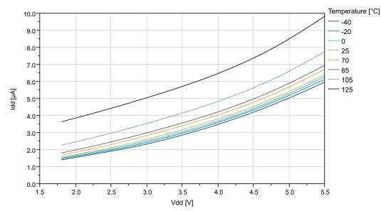
Figure 32-9. ATtiny204/ATtiny404: Idle Supply Current vs. V<sub>DD</sub> (f=32 KHz OSCULP32K)
