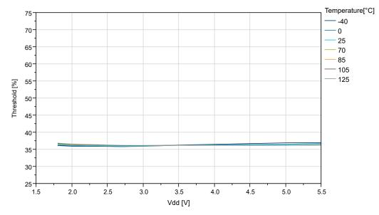
Figure 32-19. I/O Pin Input Threshold Voltage vs.  $V_{DD}$  (V<sub>IL</sub>)
