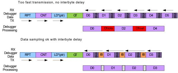
In Figure 30-18, GT denotes the Guard Time insertion, SB is for Stop Bit and IB is the inserted interbyte delay. The rest of the frames are data and instructions.
