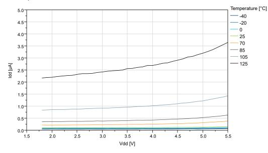
32.1.4 Supply Currents in Standby Mode for ATtiny204/ATtiny404 Figure 32-12. ATtiny204/ATtiny404: Standby Mode Supply Current vs. V<sub>DD</sub> (RTC Running with External 32 KHz Osc.)
