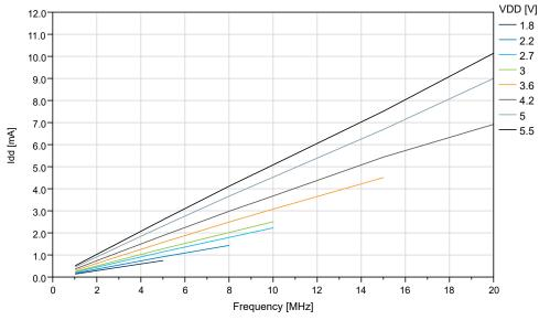
Figure 32-2. ATtiny204/ATtiny404: Active Supply Current vs. Frequency [0.1, 1.0] MHz at T=25°C
