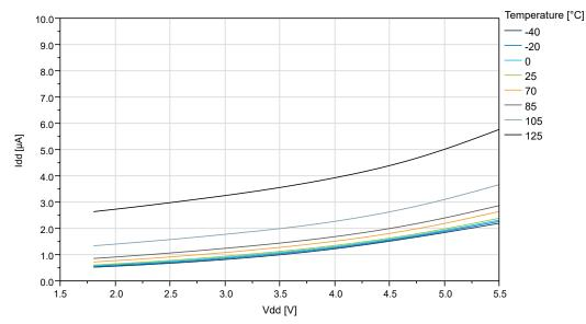
Figure 32-14. ATtiny204/ATtiny404: Standby Mode Supply Current vs. V<sub>DD</sub> (Sampled BOD Running at 125 Hz)
