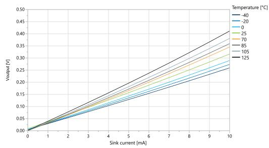
Figure 32-21. I/O Pin Output Voltage vs. Sink Current (V<sub>DD</sub>=3.0V)
