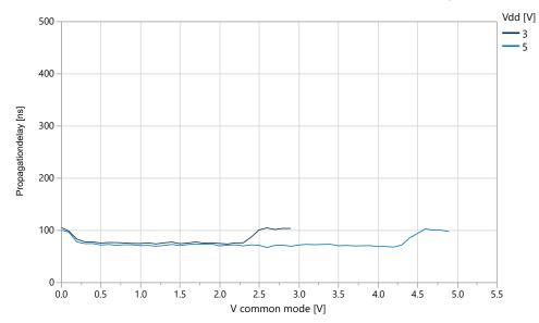
Figure 32-55. Propagation Delay vs.  $V_{CM}$  Falling Positive Input,  $V_{OD}$  = 25 mV (T=25°C)
