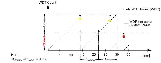
The Window mode is enabled by writing a non-zero value to the WINDOW bit field in the Control A register (WDT.CTRLA), and disabled by writing WINDOW=0x0.
