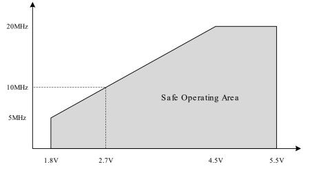
Figure 31-1. Maximum Frequency vs. V<sub>DD</sub> for [-40, 105]°C
