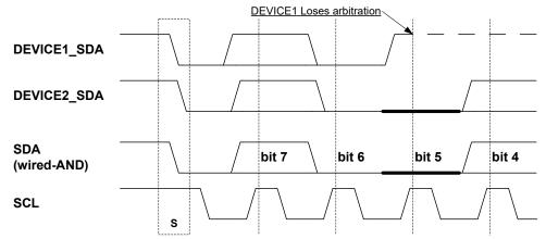
Figure 25-10 shows an example where two TWI masters are contending for bus ownership. Both devices are able to issue a Start condition, but DEVICE1 loses arbitration when attempting to transmit a high level (bit 5) while DEVICE2 is transmitting a low level.
