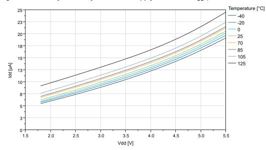
Figure 32-5. ATtiny204/ATtiny404: Active Supply Current vs. V<sub>DD</sub> (f=32 KHz OSCULP32K)
