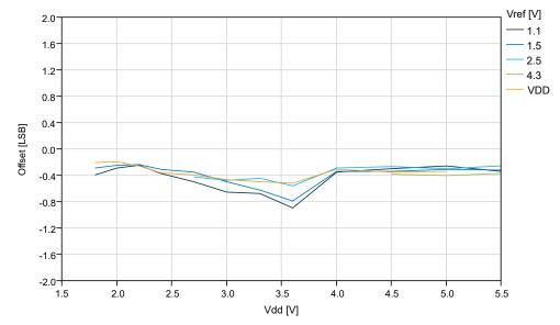
Figure 32-49. Offset Error vs.  $V_{DD}$  (f<sub>ADC</sub>=115 ksps) at T=25°C, REFSEL = Internal Reference
