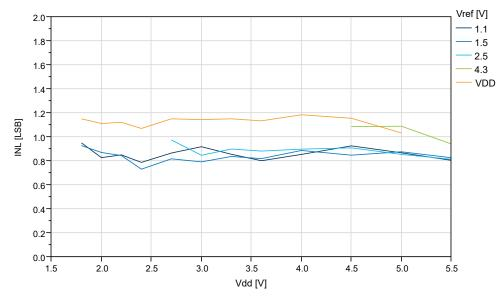
Figure 32-47. INL vs. V<sub>DD</sub> (f<sub>ADC</sub>=115 ksps) at T=25°C, REFSEL = Internal Reference
