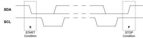
Multiple Start conditions can be issued during a single transaction. A Start condition that is not directly following a Stop condition is called a repeated Start condition (Sr).
