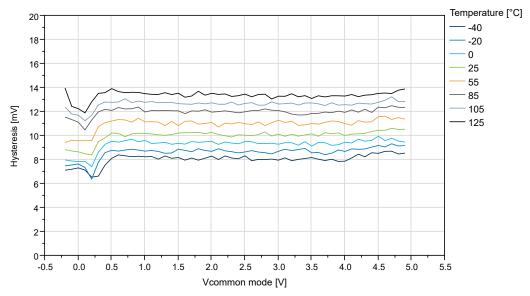
Figure 32-51. Hysteresis vs. V<sub>CM</sub> - 10 mV (V<sub>DD</sub>=5V)
