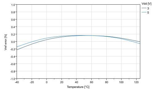
Figure 32-33. Internal 2.5V Reference vs. Temperature
