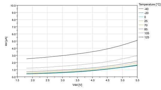
Figure 32-15. ATtiny204/ATtiny404: Standby Mode Supply Current vs. V<sub>DD</sub> (Sampled BOD Running at 1 kHz)
