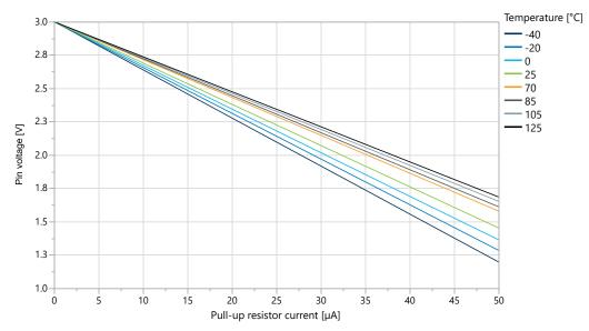
Figure 32-29. I/O Pin Pull-Up Resistor Current vs. Input Voltage (V<sub>DD</sub>=3.0V)
