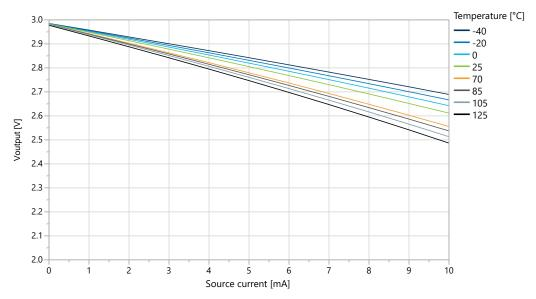
Figure 32-25. I/O Pin Output Voltage vs. Source Current (V<sub>DD</sub>=3.0V)
