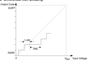
**Quantization Error** Due to the quantization of the input voltage into a finite number of codes, a range of input voltages (1 LSB wide) will code to the same value. Always ±0.5 LSB.
