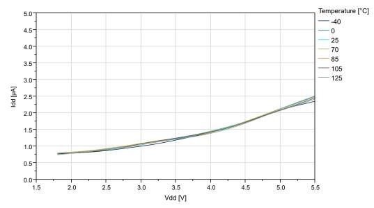
Figure 32-37. BOD Current vs. V<sub>DD</sub> (Sampled BOD at 1 kHz)
