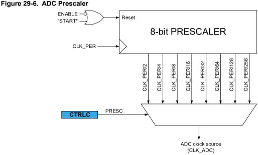
The ADC requires an input clock frequency between 50 kHz and 1.5 MHz for maximum resolution. If a lower resolution than 10 bits is selected, the input clock frequency to the ADC can be higher than 1.5 MHz to get a higher sample rate.
