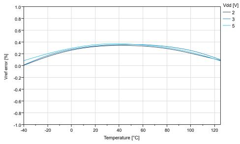
Figure 32-31. Internal 0.55V Reference vs. Temperature
