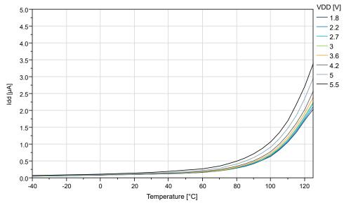
Figure 32-11. ATtiny204/ATtiny404: Power-Down Mode Supply Current vs. V<sub>DD</sub> (All Functions Disabled)
