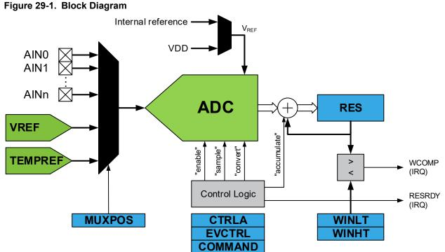
The analog input channel is selected by writing to the MUXPOS bits in the MUXPOS register (ADC.MUXPOS). Any of the ADC input pins, GND, can be selected as single-ended input to the ADC. The ADC is enabled by writing a '1' to the ADC ENABLE bit in the Control A register (ADC.CTRLA). Voltage reference and input channel selections will not go into effect before the ADC is enabled. The ADC does not consume power when the ENABLE bit in ADC.CTRLA is '0'.
