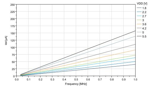
Figure 32-7. ATtiny204/ATtiny404: Idle Supply Current vs. Low Frequency (0.1-1.0 MHz) at T=25°C
