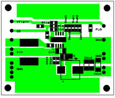
(The broad land of Lx section enables a connection with large inductors and diodes).
