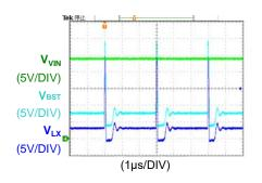
R1243x001A/R1243x001B, R1243S001E (R1243K001A, V<sub>IN</sub> = 24 V, V<sub>OUT</sub> = 5.0 V, L = 4.7 μH, C<sub>OUT</sub> = 10 μF, R<sub>OUT</sub> = 5.0 Ω (I<sub>OUT</sub> = 1.0 A), Ta = 25°C)
