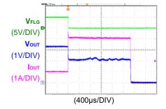
17) Fold-back Operation Waveform R1243x001B/R1243x001D (R1243S001D, V<sub>IN</sub> = 12 V, V<sub>OUT</sub> = 5.0 V, L = 10 μH, C<sub>OUT</sub> = 22 μF, R<sub>OUT</sub> = 5.0 Ω→0.5 Ω, Ta = 25°C)
