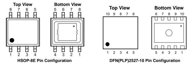
\* The tab is substrate level (GND). It must be connected to the GND level.
