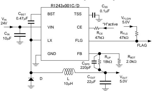
V<sub>OUT</sub> = 5.0 V, t<sub>SS</sub> = 12 ms, Flag Function Using
