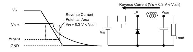
Fig. 6 Shutdown Using Input Voltage Control
