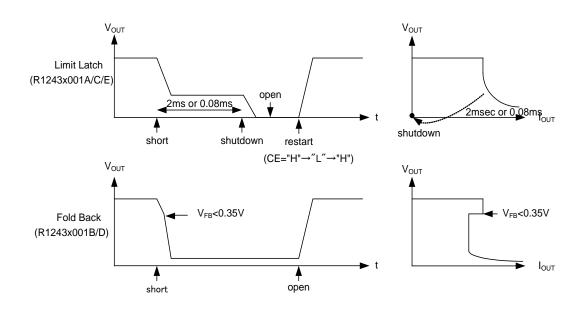
Fig. 5 LX Current Limit Sequencing
