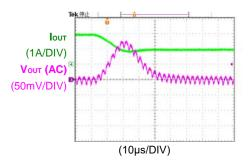
14) Switching Operation Waveform R1243x001A/R1243x001B, R1243S001E (R1243K001A,  $V_{IN} = 24 V$ ,  $V_{OUT} = 5.0 V$ , L = 4.7  $\mu$ H, C<sub>OUT</sub> = 10  $\mu$ F, I<sub>OUT</sub> = 0 mA, Ta = 25°C)
