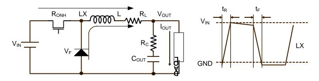
Nch High-side Tr. Turn-on Loss:  $P_{ON} = R_{ONH} \times I_{OUT}^2 \times Onduty$
