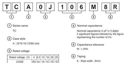
R : Positive electrode on the side opposite to sprocket hole
