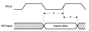
Figure 5-48. PCI Input Timing (33-/66-MHz)
