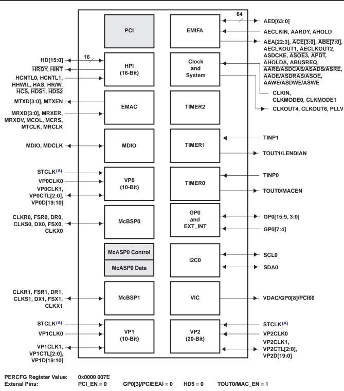
Shading denotes a peripheral module not available for this configuration.
