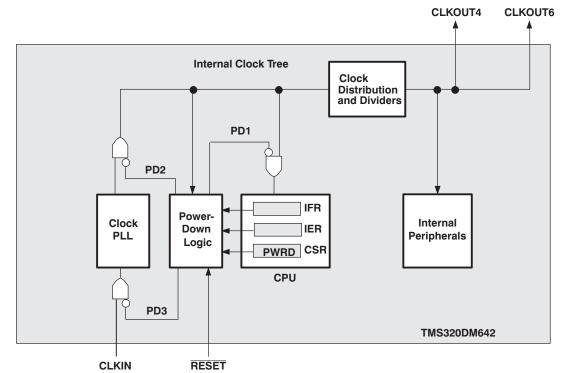
A. External input clocks, with the exception of CLKIN, are not gated by the power-down mode logic.
