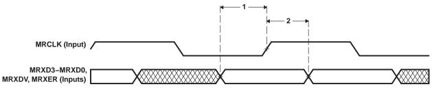
Figure 5-65. EMAC Receive Interface Timing
