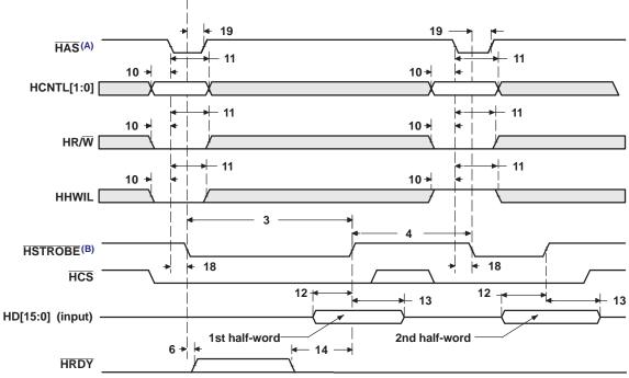
A. For correct operation, strobe the HAS signal only once per HSTROBE active cycle.
