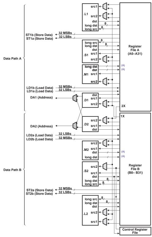
A. For the .M functional units, the long dst is 32 MSBs and the dst is 32 LSBs.
