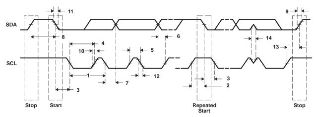
Figure 5-36. I2C Receive Timings
