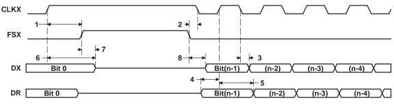
Figure 5-55. McBSP Timing as SPI Master or Slave: CLKSTP = 10b, CLKXP = 1
