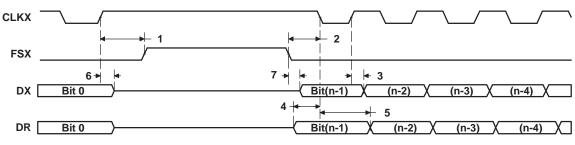
Figure 5-56. McBSP Timing as SPI Master or Slave: CLKSTP = 11b, CLKXP = 1
