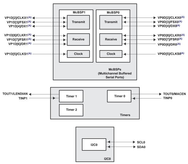
A. These McBSP1 and McBSP0 pins are muxed with the Video Port 1 (VP1) and Video Port 0 (VP0) peripherals, respectively. By default, these signals function as VP1 and VP0, respectively. For more details on these muxed pins, see the Device Configurations section of this data sheet.
