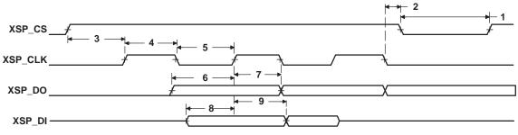
Figure 5-50. PCI Serial EEPROM Interface Timing
