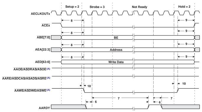
A. AAOE/ASDRAS/ASOE, AARE/ASDCAS/ASADS/ASRE, and AAWE/ASDWE/ASWE operate as AAOE (identified under select signals), AARE, and AAWE, respectively, during asynchronous memory accesses.
