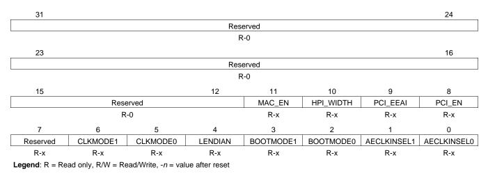
Figure 3-5. Device Status Register (DEVSTAT) Description - 0x01B3 F004
