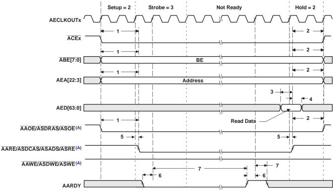
A. AAOE/ASDRAS/ASOE, AARE/ASDCAS/ASADS/ASRE, and AAWE/ASDWE/ASWE operate as AAOE (identified under select signals), AARE, and AAWE, respectively, during asynchronous memory accesses.
