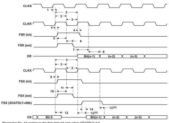
Parameter No. 13 applies to the first data bit *only* when XDATDLY  $\neq$  0.
