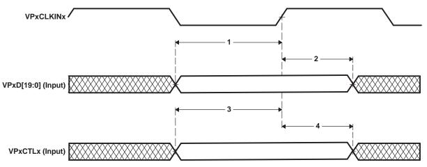
Figure 5-58. Video Port Capture Data and Control Input Timing
