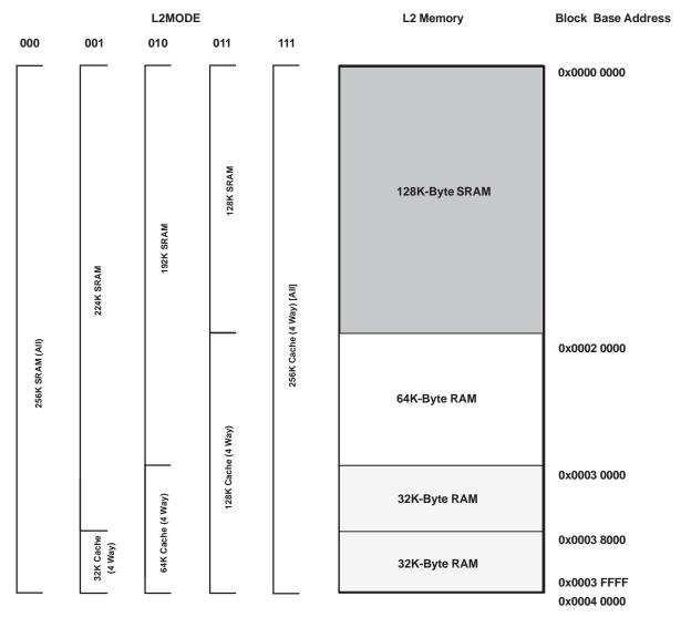
Figure 2-2. TMS320DM642 L2 Architecture Memory Configuration
