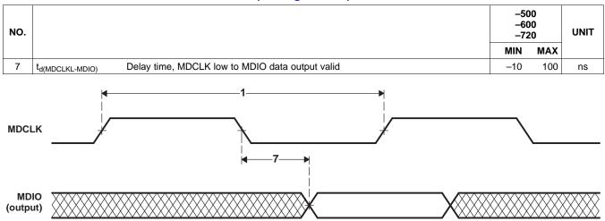
Figure 5-68. MDIO Output Timing
