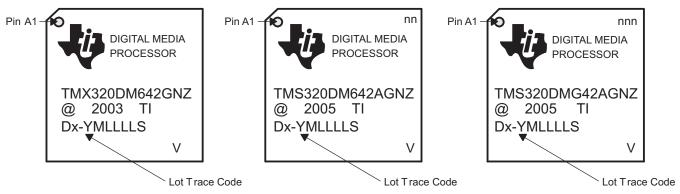
Figure 6-1. Example, Lot Trace Codes for TMX320DM642 and TMS320DM642 (GDK and GNZ Packages)
