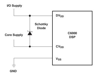
Figure 5-5. Schottky Diode Diagram
