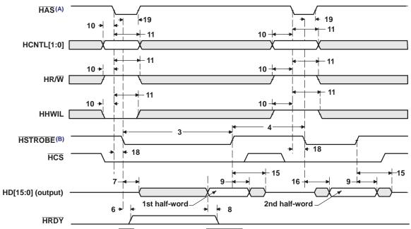
A. For correct operation, strobe the HAS signal only once per HSTROBE active cycle.
