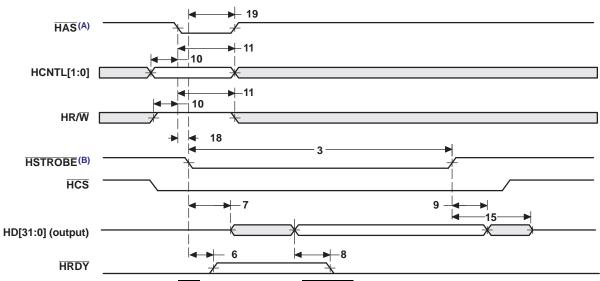
A. For correct operation, strobe the HAS signal only once per HSTROBE active cycle.
