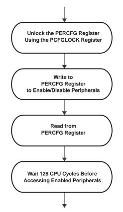
Figure 3-3. Peripheral Enable/Disable Flow Diagram
