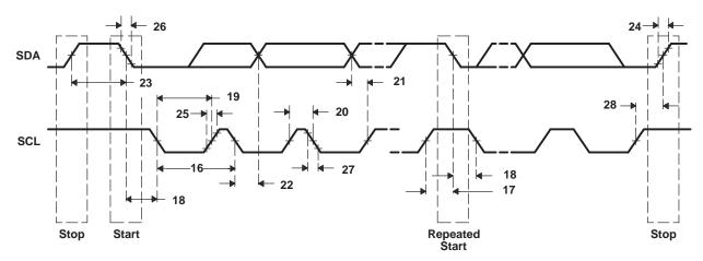
Figure 5-37. I2C Transmit Timings
