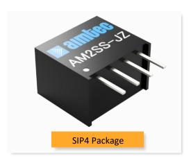
The AM2SS-JZ is a 2W SIP4 DC/DC converter that offers great cost savings thanks to an improved manufacturing process. It also features excellent reliability and performance while offering a standard input voltage range of 5VDC as well as an output voltage of 5-24V. This compact SIP4 design will surely benefit your new system design.
