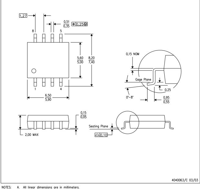
A. All linear dimensions are in millimeters.
