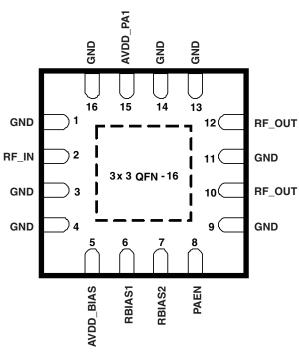
Figure 1. CC2595 Pinout
