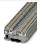
Feed-through terminal block, Connection method: Push-in connection, Cross section: 0.14 mm² - 1.5 mm², AWG: 26 - 16, Width: 3.5 mm, Height: 30.5 mm, Color: red, Mounting type: NS 35/7,5, NS 35/15
