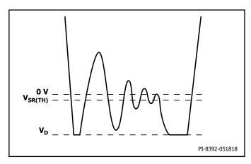
Figure 10. Unacceptable FORWARD Pin Waveform After Handshake with SR Switch Conduction During Flyback Cycle.
