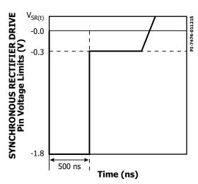
Figure 25. SYNCHRONOUS RECTIFIER DRIVE Pin Negative Voltage.
