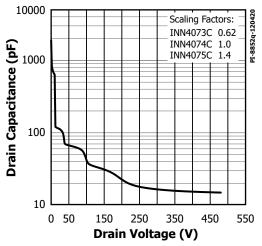
Figure 22.  $C_{OSS}$  vs. Drain Voltage.
