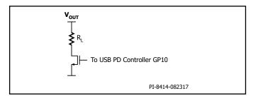
Figure 9. Active Pre-Load Circuit.
