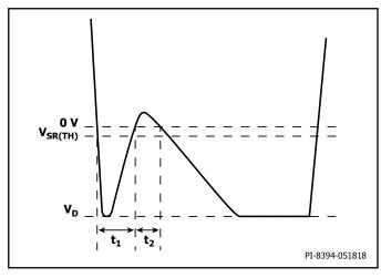
Figure 12. Unacceptable FORWARD Pin Waveform Before Handshake with Body Diode Conduction During Flyback Cycle.
