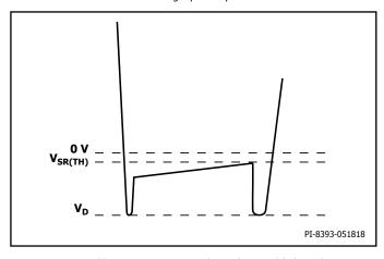
Figure 11. Acceptable FORWARD Pin Waveform After Handshake with SR Switch Conduction During Flyback Cycle.
