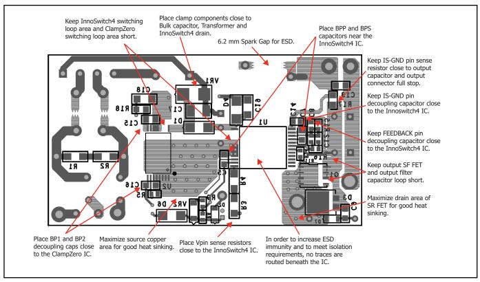
Figure 17. PCB Layout Bottom Side.
