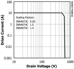
Figure 24. Maximum Allowable Drain Current vs. Drain Voltage.
