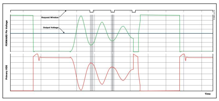
Figure 7. Intelligent Zero Voltage Switching.
