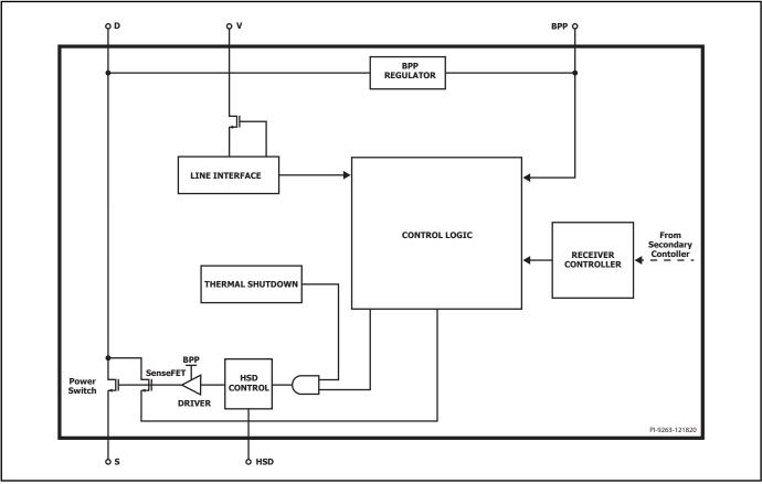
Figure 3. Primary Controller Block Diagram.
