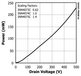
Figure 23. Drain Capacitance Power.
