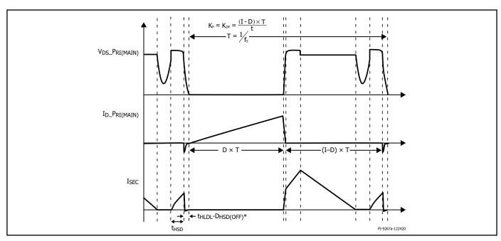
Figure 18. Discontinuous Conduction Mode Current Waveform at High-Line,  $K_p > 1$ . \*D<sub>HSD(OFF)</sub> is delay from HSD low to ClampZero OFF, please refer to ClampZero data sheet.
