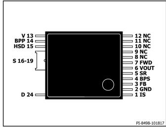
Figure 5. Pin Configuration.
