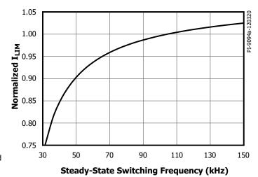
Figure 6. Normalized Primary Current vs. Frequency.
