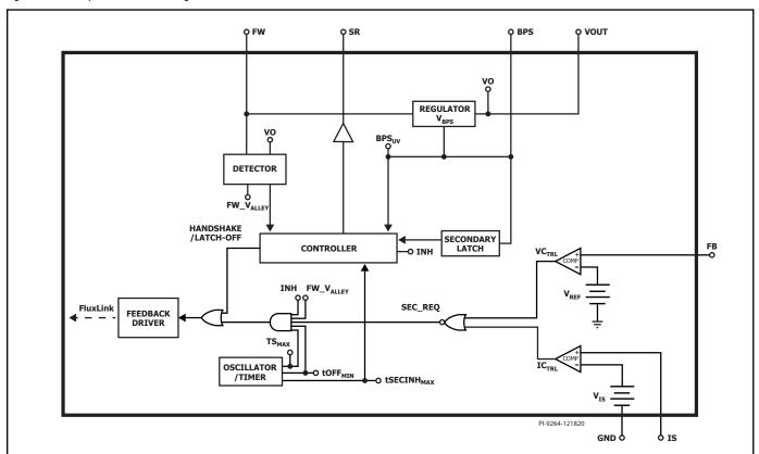
Figure 4. Secondary Controller Block Diagram.
