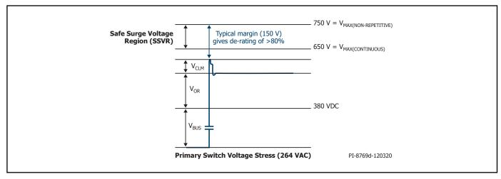
Figure 20. Peak Drain Voltage for 264 VAC Input Voltage.
