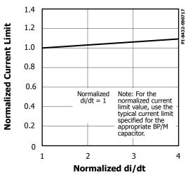
Figure 26. Standard Current Limit vs. di/dt.
