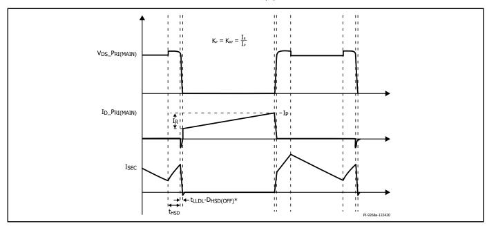
Figure 19. Continuous Conduction Mode Current Waveform at Low-Line,  $K_p < 1$ . \*D<sub>HSD(OFF)</sub> is delay from HSD low to ClampZero OFF, please refer to ClampZero data sheet.
