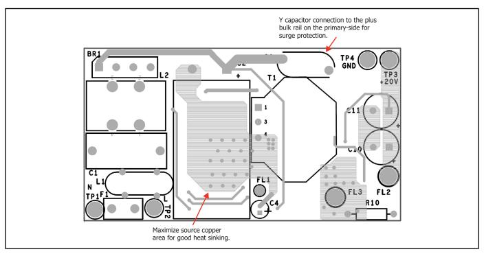
Figure 16. PCB Layout Top Side.
