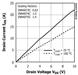
Figure 21. Output Characteristics.
