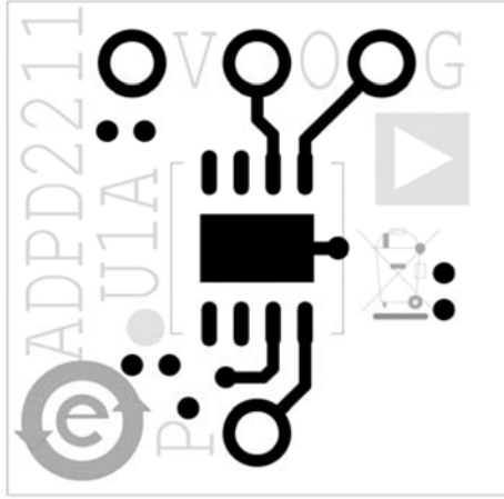
Figure 15. ADPD2211 Evaluation Board Top Layer
