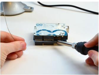
Now from above, solder the two end pins a stacky header to the PCB. You don't have to do a great job soldering, just make sure it's tacked together.
