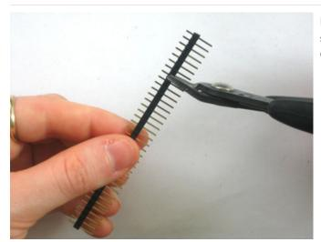
Next its time to make the male headers from the long strip. use diagonal cutters or pliers to clip off 4 parts, one 6-pin, two 8-pin, and one 10-pin
