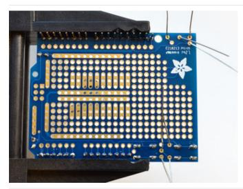
Bend out the leads of the LEDs and resistors so they sit flat againt the  $\ensuremath{\mathsf{PCB}}$
