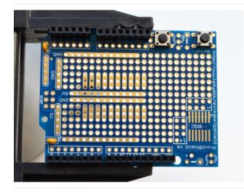
Snap the two buttons into the top corner of the PCB. They will snap into place and sit flat against the PCB. They are symmetric so you can insert them 'either way'
