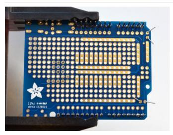
Bend the two little capacitor leads out so that you can flip over the PCB without the caps falling out
