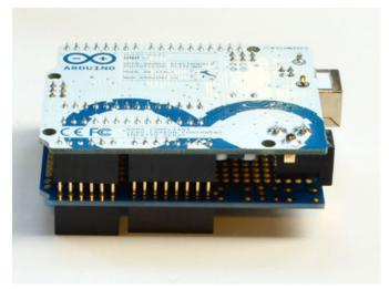
Flip over the Arduino and place it flat on the table so that the PCB sits flat against the stacky headers and the stacky headers are flat against the table
