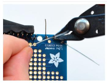
Clip all the leads down so that the long wires are no longer than the solder points
