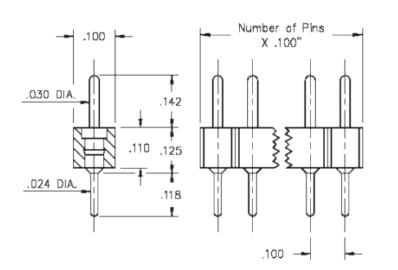
Description: Interconnect Header Low Profile Solder Tail Header .030" (0,76mm) Pin Head Single Row Through Hole Plating Code: 90 Shell Plating: 200 µ" Tin/Lead(93/7) over 100 µ" Nickel
