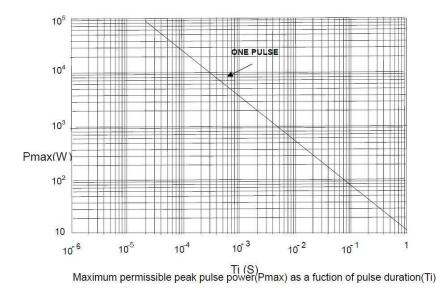
Condition test: Resistance change  $\leq \pm \%$  with pulse 1000 cycles as like the figure.(Reference Only) 1. Added power and added voltage are within the lower teritory of this graph. 2. Added in normal temperature and humidity.
