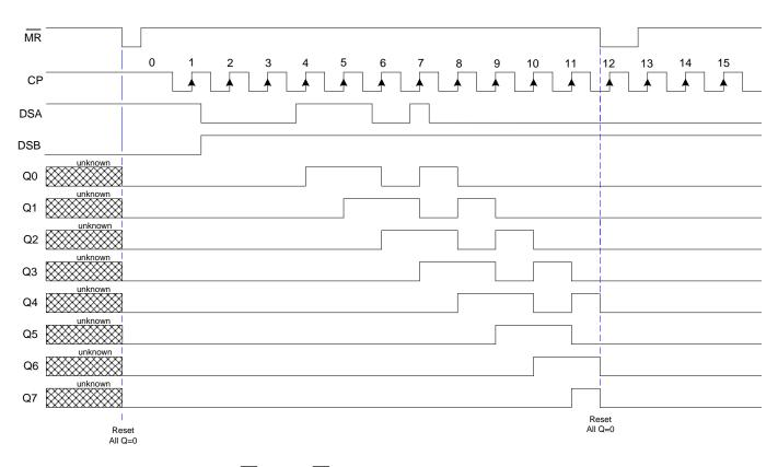
Notes: 5. All Q values are reset to LOW when MR goes low. MR is asynchronous and overrides all other signals. 6. Serial data supplied at DSA and DSB is ANDED and transferred to Q0 on positive edge of CP.
