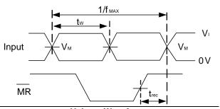
Voltage Waveform Pulse Duration and Recovery Time
