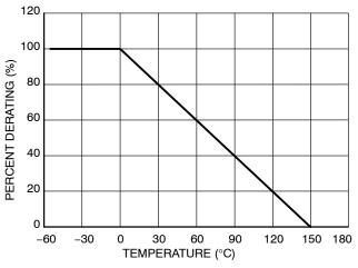
Figure 6. Temperature Power Dissipation Derating
