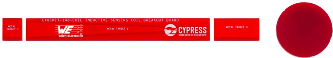
Figure 2-3. Metal Targets on the CY8CKIT-148-COIL
