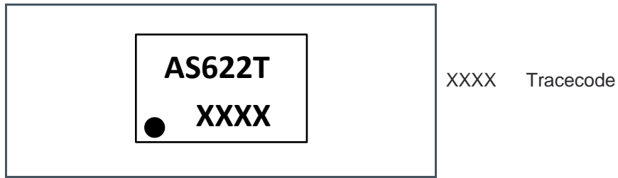
Figure 40: WLCSP Package Marking/Code for AS6221T
