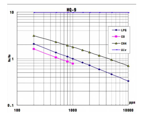
According to the figure, we can see that the minimum concentration we can test is 200ppm and the maximum is 10000ppm, in a other word, we can get a concentration of gas between 0.02% and 1%. However, we can't provide a formula because the relation between ratio and concentration is nonlinear.
