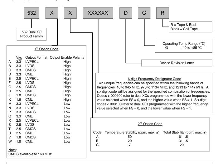
Example Part Number: 532AB000108DGR is a  $5 \times 7$  mm Dual XO in a 6 pad package. Since the six digit code (000108) is > 000100, f0 is 644.53125 MHz (lower frequency) and f1 is 693.48299 (higher frequency), with a 3.3 V supply, LVPECL output, and Output Enable active high polarity. Temperature stability is specified as  $\pm 20$  ppm. The part is specified for a -40 to  $\pm 40$  to  $\pm 40$  c ambient temperature range operation and is shipped in tape and reel format.
