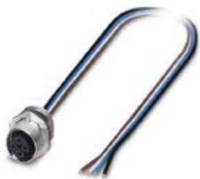
Flush-type connector, Universal, 4-position, Socket, straight, M12-SPEEDCON, A-coded, Front mounting, M16 x 1.5, Individual wires, cable length: 0.5 m, 0.34 mm 2 , TPE litz wire
