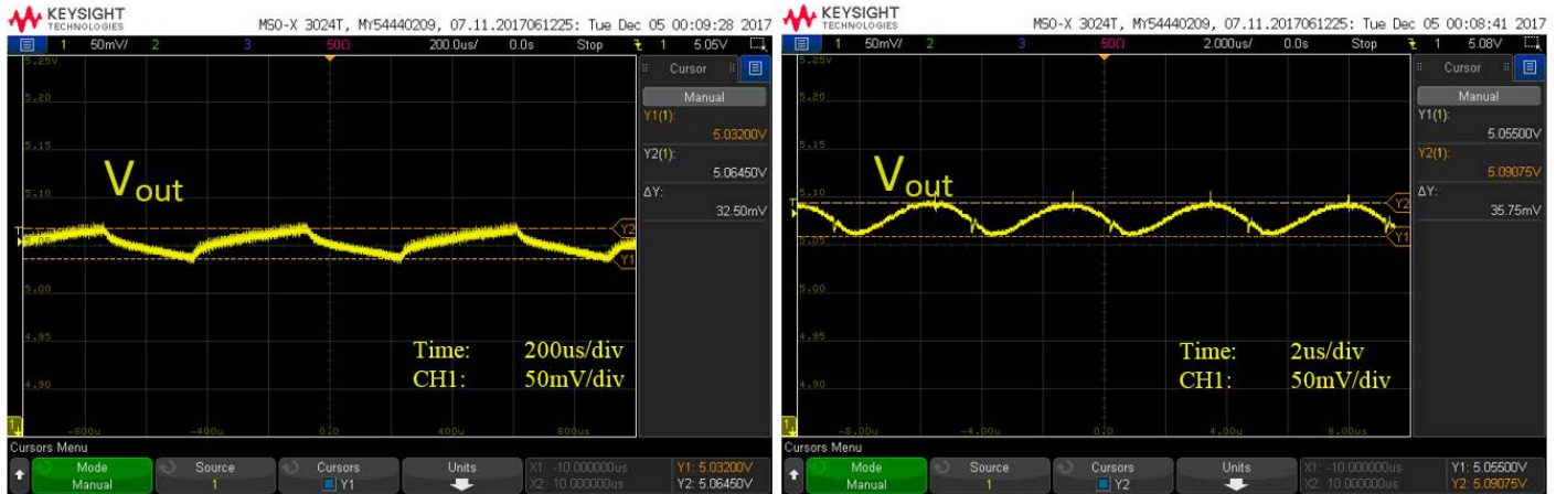
Figure 7.1. Si3406-Non-Isolated Flyback C3 EVB Output Voltage Ripple No Load (Left) and Heavy Load (Right) Conditions
