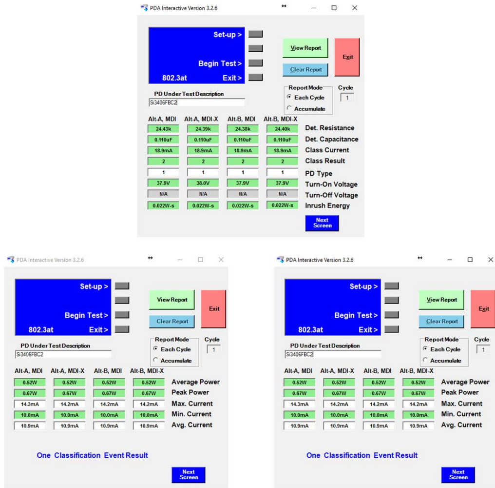
Figure 4.1. Si3406 Non-Isolated Flyback PD SIFOS PoE Compatibility Test Results
