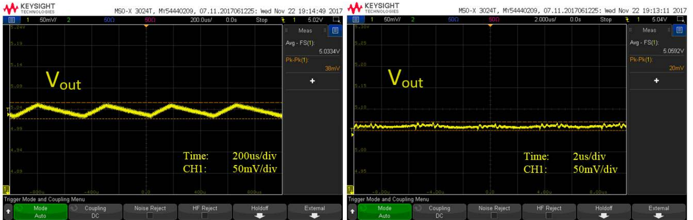
Figure 7.1. Si3406 Non-Isolated Flyback EVB Output Voltage Ripple No Load (Left) and Heavy Load (Right) Conditions
