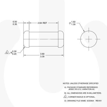
Figure 1. 2-TERMINAL, SOD-80, JEDEC DO-213AC, MINI-MELF
