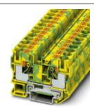
Ground modular terminal block, Connection method: Push-in connection, Cross section: 0.5 mm² - 16 mm², AWG: 20 - 6, Width: 10.2 mm, Height: 49.5 mm, Color: green-yellow, Mounting type: NS 35/7,5, NS 35/15
