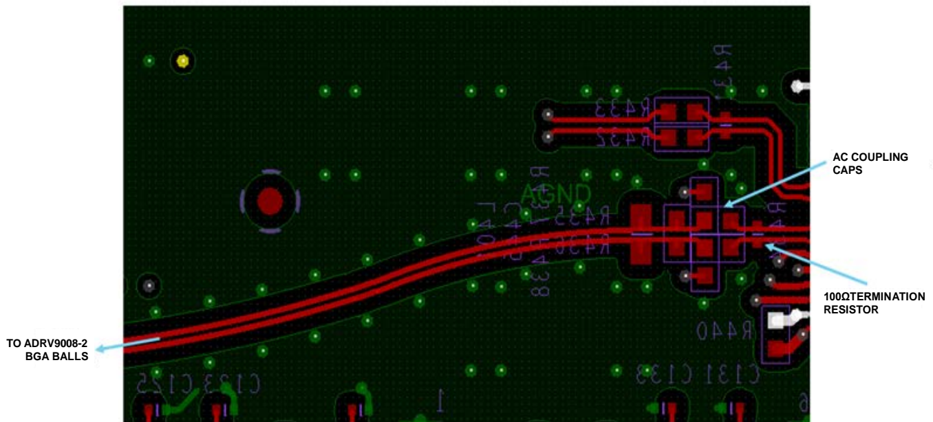
Figure 272. REF_CLK_IN \pm Routing Recommendation
