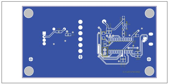
Figure 7. MAX31865 EV Kit PCB Layout—Bottom
