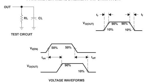
Figure 1. Test Circuit and Voltage Waveforms
