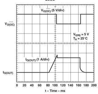
Figure 7. TPS2032, Ramped Load on Enabled Device
