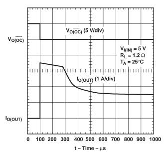
Figure 8. 2.6-Ω Load Connected to an Enabled TPS2032 Device
