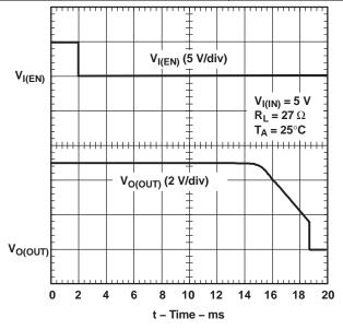
Figure 3. Turnoff Delay and Fall Time
