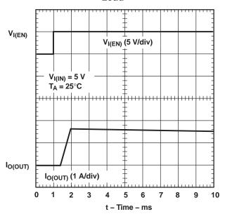
Figure 6. Device Enabled Into Short
