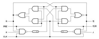
Figure 4. Logic Diagram, Each Flip-Flop (Positive Logic)
