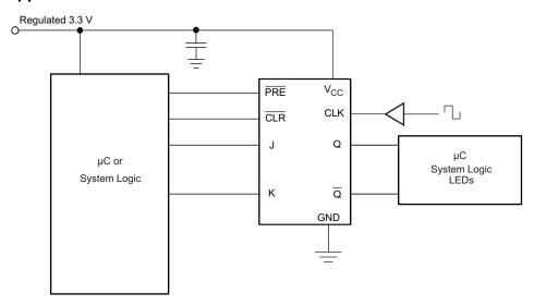
Figure 5. Typical Application Schematic
