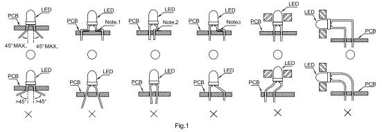
"Correct mounting method "X" Incorrect mounting method
