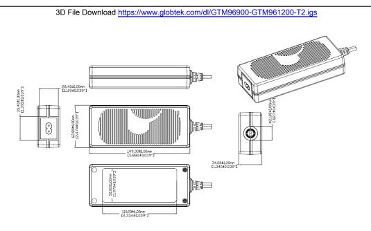
Alternative housing with input cord clamp to prevent accidental removal of the power cord. Product PN# ends with suffix "CL"
