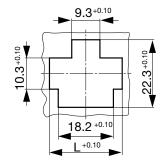
Pannel thickness s length L 0.8 mm 24.0 mm 24.6 mm 1.0 mm 25.2 mm 1.2 mm 26.2 mm 1.6 mm
