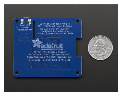
Comes as one fully assembled and tested DPI Kippah circuit board. You may need a soldering iron to adjust the backlight by soldering closed a PCB jumper (check the tutorial on this). TFT display (https://adafru.it/Cfx), USB micro-B cable (http://adafru.it/592), FPC extension cable (https://adafru.it/eVZ), bent wire stand (https://adafru.it/d7M), and Raspberry Pi not included (but we do carry them in the shop!)
