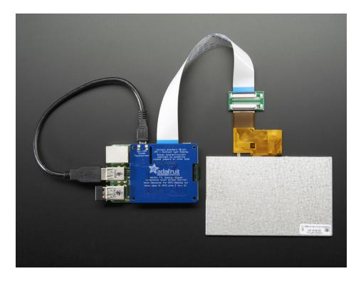
OK so, exciting right? But, what's the catch? The catch is **this add on board uses nearly every pin available on the Raspberry Pi and those pins are hardcoded, they cannot be moved or rearranged**. The pins used are GPIO 2 through 21 inclusive. That means you don't get the UART RX/TX pins (no console cable) and you don't get the standard user I2C pins, the EEPROM I2C pins, or hardware SPI pins. You do get to use pins #22, #23, #24, #25, #26 and #27, and the USB ports are fine to use too.
