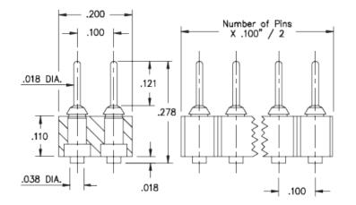
**Description:** Interconnect Header Surface Mount Pin Header .018" (0,46mm) Pin Head Double Row Surface Mount **Plating Code:** 10 Shell Plating: 10 µ" Gold over 100 µ" Nickel
