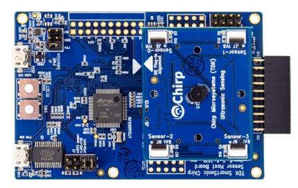
Part of the SmartSonic platform, the DK-CH101 is designed around Atmel's SAMG55 Cortex-M4 MCU, and can be used by developers for rapid evaluation and development of CH-101 based solutions. The DK-CH101 includes an on-board Embedded Debugger so external tools are not required to program or debug the SAMG55 MCU. The DK-CH101 includes an on-board Embedded Debugger so external tools are not required to program or debug the SAMG55 MCU.
