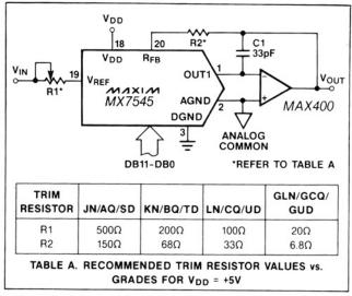
Figure 3. Unipolar Binary Operation
