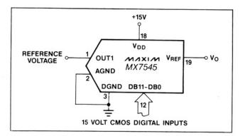
Figure 5. Single Supply Operating Using Voltage Switching Mode
