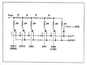
Figure 1. Simplified D/A Circuit of MX7545
