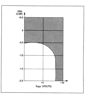
Figure 7. Differential Nonlinearity vs. Reference Voltage for Figure 4 Circuit.  $V_{DD}$  = 15 Volts. Shaded Area Shows Range of Values of Differential Nonlinearity that Typically Occur for L, C, and U Grades.
