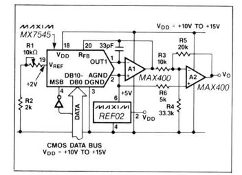
Figure 8. Single Supply "Bipolar" 2's Complement D/A Converter
