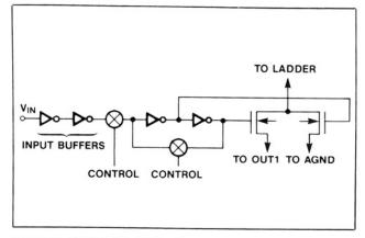
Figure 2. Digital Input Structure
