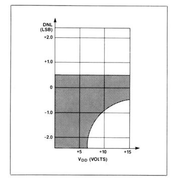
Figure 6. Differential Nonlinearity vs.  $V_{DD}$  for Figure 4 Circuit. Reference Voltage = 2.5 Volts. Shaded Area Shows Range of Values of Differential Nonlinearity that Typically Occur for L, C and U Grades.
