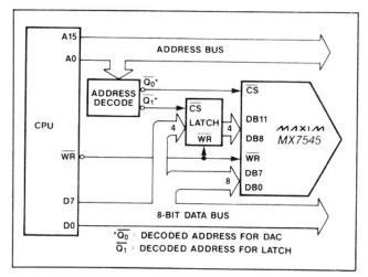
Figure 9. 8-Bit Processor to MX7545 Interface
