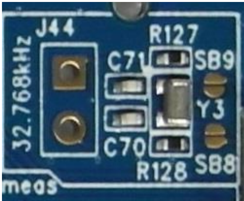
Figure 21: Optional external 32.768kHz crystal circuit schematic and PCB
