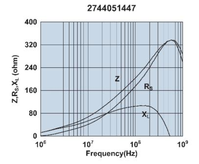
Impedance, reactance, and resistance vs. frequency.
