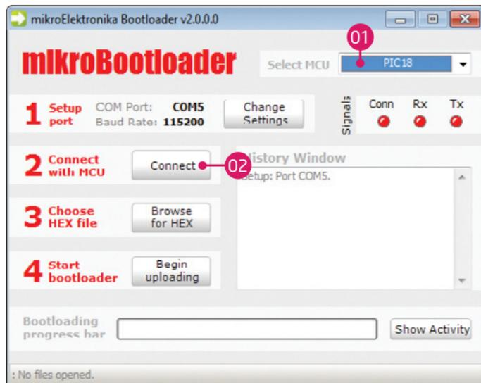
Figure 1-4: Connecting mikromedia with mikroBootloader
