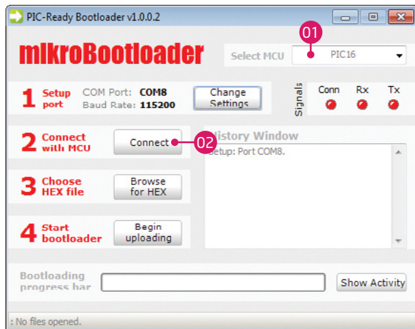
Figure 1-4: Connecting Ready for PIC with mikroBootloader
