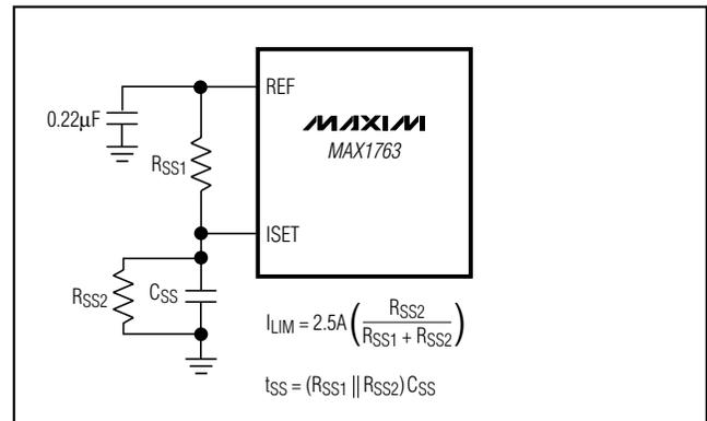
Figure 8. Soft-Start with Reduced Switch Limit Current
