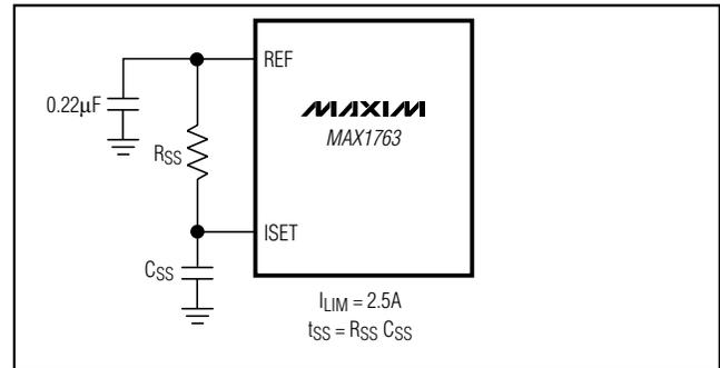
Figure 7. Soft-Start with Maximum Switch Limit Current
