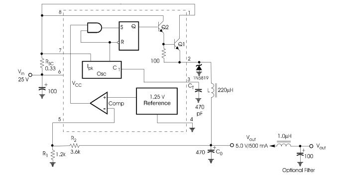
Fig.3. Step-down Converter
