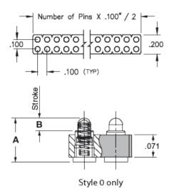
**Description:** Interconnect SLC Header Spring-Loaded Header Vertical Mount SMT Double Row Surface Mount **Plating Code:** Shell Plating:  $20\mu$ " Gold over  $100\mu$ " Nickel Inner Spring Plating: 10μ" Gold Packaging: Packaged in Bulk
