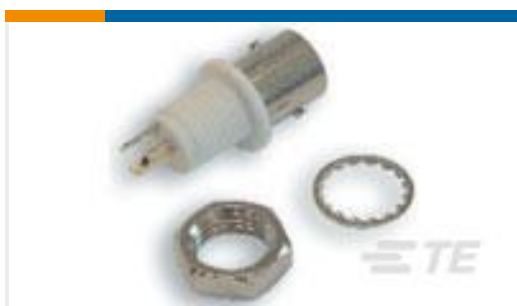
TE Part #1-1337448-0 BNC BHSkt + TAG 50Ohm Nickel Pltd
